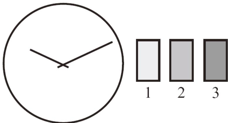
**Important:** never make a fast date change when the watch indicates a time between 9 p.m. and 3 a.m. This might damage the mechanism.
